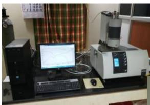
Simultaneous Thermal Analyser (STA)
